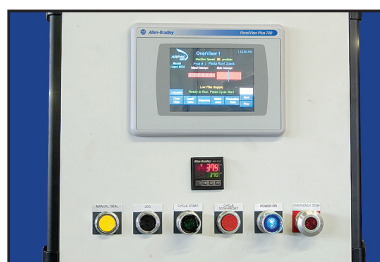
Optional Operator Controls Can Be Reached From Both Sides of Machine
